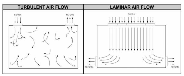
Isokinetic sampling is required in laminar flow (aka unidirectional flow) areas.
