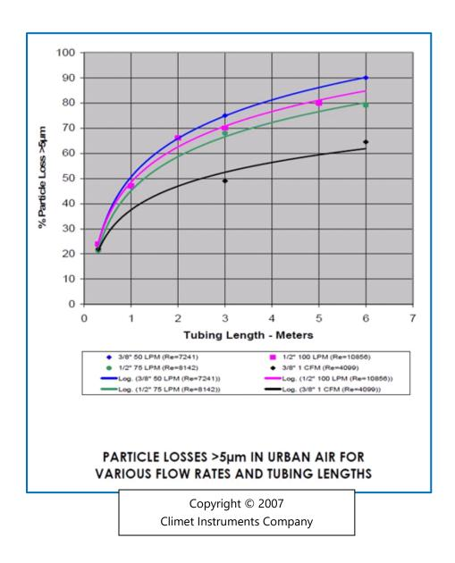
As a consequence of Climet validation procedures, Climet recommended a shorter transport tubing length for a 100 LPM particle counter of 2 meters (~6 feet) maximum.
